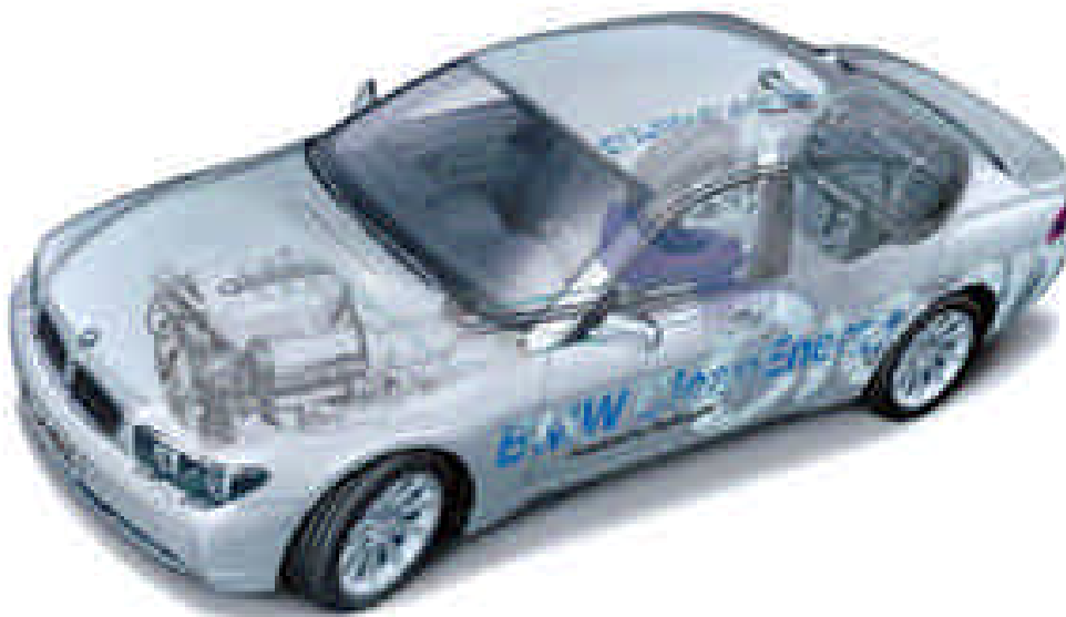
BMW 7 series with internal combustion engine using LH2
