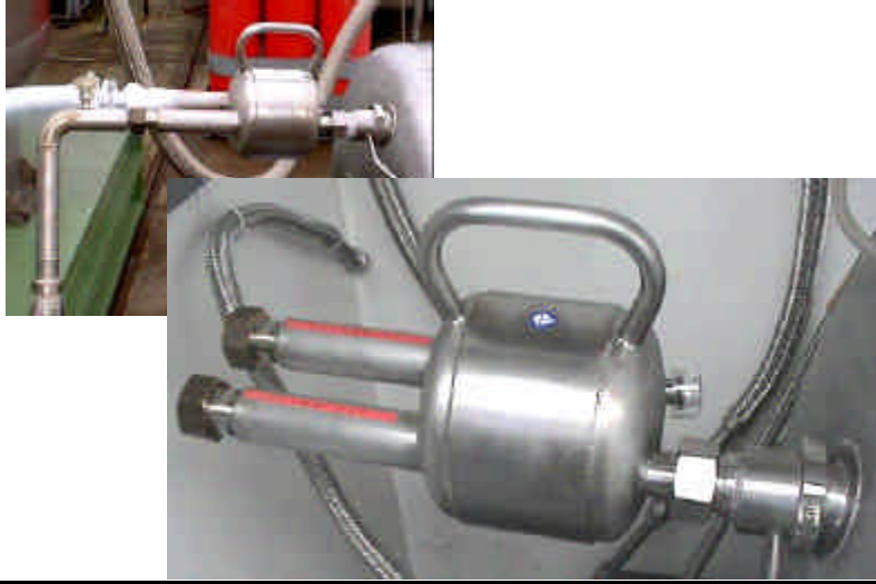
Fig. 3: Filling adapter for 2-flow interface
